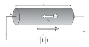
Consider a conductor of length  $\ell$  and area of cross section A connected to battery of potential difference V. Then, volume of the conductor is  $A\ell$ . If number density of electrons in the conductor
