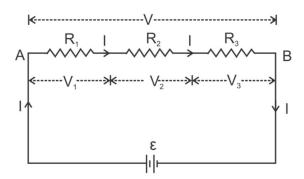
Since current measures the rate of flow of charge, this means that the same current I flows through  $R_1$  and  $R_2$ . By Ohm's law:
