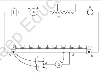
Two cells whose emfs are to compared are connected as shown in the figure. First connect terminal 1 with terminal 3 such that cell with emf  $\epsilon_1$  comes in the circuit. If  $\ell_1$  is the balancing length in this case, we can write
