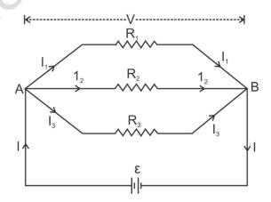
The currents  $I_1I_1$ ,  $I_2$  and  $I_3$  shown in the figure are the rates of flow of charge at the points indicated. Hence,
